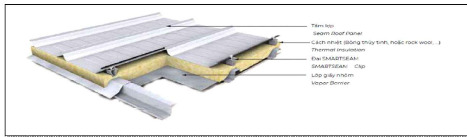
METAL ROOF SHEET - SEAMLOCK THK 0.45MM
